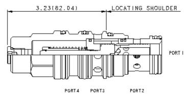
The direct-acting reducer/reliever main section is meant to act as an interface between a low flow pressure source at port 4 and a circuit with higher flow requirements. The valve will reduce a high primary pressure at the inlet (port 2) to a reduced pressure at port 1, with a full-flow relief function from port 1 to tank (port 3).
