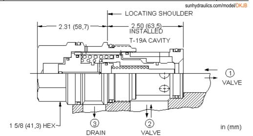
This is a normally closed, balanced poppet, switching element. When port 3 is blocked, the poppet remains in the closed position. Venting port 3 shifts it to the open position, provided there is sufficient pressure at port 2.
