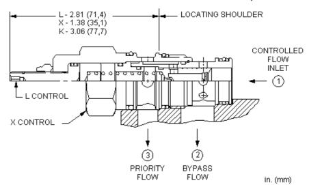
This valve is a modification of an FRDA. It controls flow in the bypass mode only. If the bypass pressure exceeds the pressure at the priority port the priority flow will no longer be pressure compensated. This modification was done in an attempt to improve system stability in specific cases.
