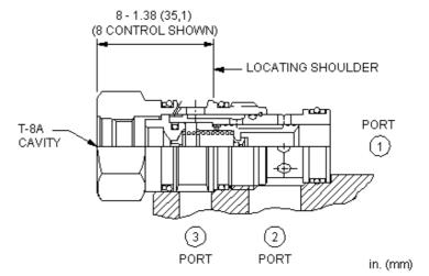
This valve is a, 3-way directional cartridge (1 blocked, 2 to 3 open) that incorporates an integral pilot control cavity. It may be used by itself or to actuate larger pilot-operated directional cartridges or logic elements. The valve shifts when there is flow through the pilot control cartridge installed in the T-8A cavity.
