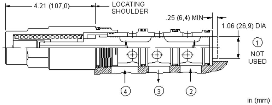
High-side shuttle cartridges are most often used in full-time regeneration circuits. When both work ports (ports 2 and 4) are at equal pressures the valve is spring-centered to an all-ports-blocked position. When one of the work ports (port 2 or 4) sees a higher pressure it is connected to the common port (port 3).
