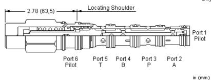
This valve is a 4-way, 3-position proportional directional valve. Work ports 2 and 4 are drained to 5 in the center position and port 3 is closed. Pilot pressure at port 1 opposes the spring and creates a variable metering orifice between ports 3 and 4 that is proportional to the pressure at 1. Piloting 6 opens 3 to 2. The force balance of the flow forces, spring and pilot pressure results in a degree of partial self-compensation as the load pressure changes.
