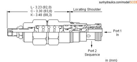
Atmospherically referenced, direct-acting sequence valves with reverse-flow check will supply a secondary circuit with flow once the pressure at the inlet (port 1) has exceeded the valve setting. Additionally, these valves incorporate an integral check valve to provide reverse flow from port 2 (sequence) to port 1 (inlet). The pressure setting of this sequence valve controls the pressure at port 1 relative to the atmospheric vent.
